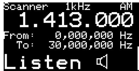
Pi Pico RX provides a scan feature, the scan feature can be accessed as a separate “home screen view”. (Different views can be selected by pressing the “back” button on the home screen.
