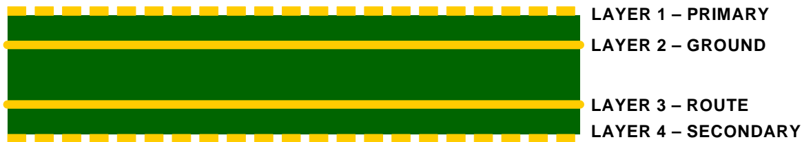
Figure 7. Four Layer Stackup
